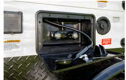
Above: Outdoor hot & cold shower Below: Spare tire, LP tank, battery disconnect
